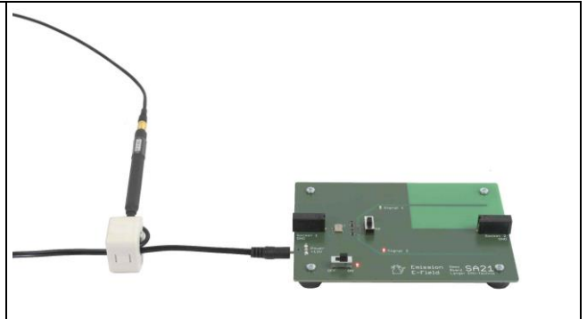
Figure 28: Using a ferrite core for the RF current measurement
